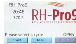
The countdown timer is initiated at the start of the sterilization cycle with “Unwrapped instruments”, “Wrapped instruments”, “Handpiece instruments”, “Wrapped cassattes” (cycles of 6, 12, 8, and 12 minutes, respectively once chamber temperature has reached 375°F). At the end of the sterilization cycle, the screen displays “CYCLE COMPLETE” in green with audible notification and the door is unlocked for instrument tray removal.
