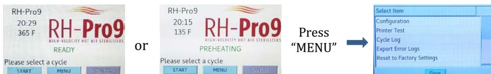
Press “Cycle Log’ to select which cycles to be saved to the flash drive as sequenced:
