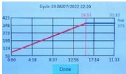
Pressing "Display records" will graphically display selected sterilization cycle. This display will not be transferred to the flash drive.
